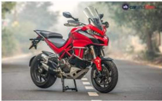
Fig 4- Ducati Multistrada 1200 S with DSS Semi active suspension system.
