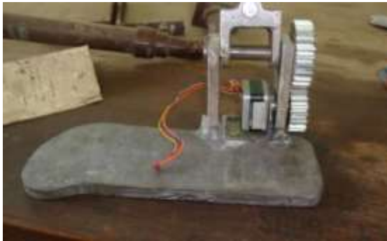
Fig 2.7: Fabricated ankle foot orthotic device.
