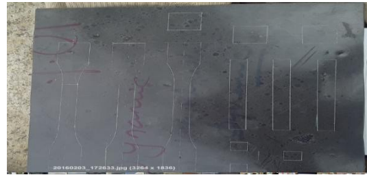
Fig. 2 Hybrid composite material using coconut ash
