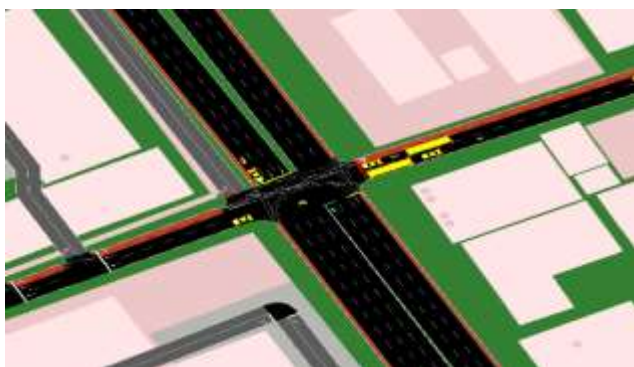
Figure 1.8.2 Simulation along Padre Faura Street and Taft Avenue intersection with bicycle lane
