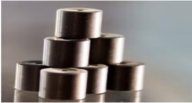
Fig 2.4: Nuclear Fuel in Pellet Form
