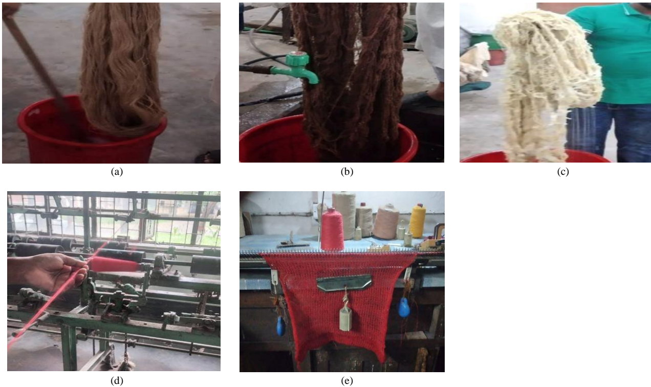
Figure 2: Different stages of yarn processing- (a) Scouring of jute yarn, (b) washing of scoured jute yarn, (c) Bleaching of jute yarn, (d) Creeling and coning, (e) Dyed jute yarn knitting.
