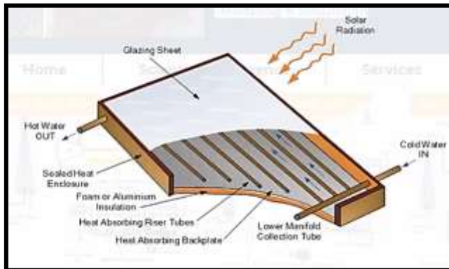
Fig 1.10: Glazed Flat Plate Solar Collector
