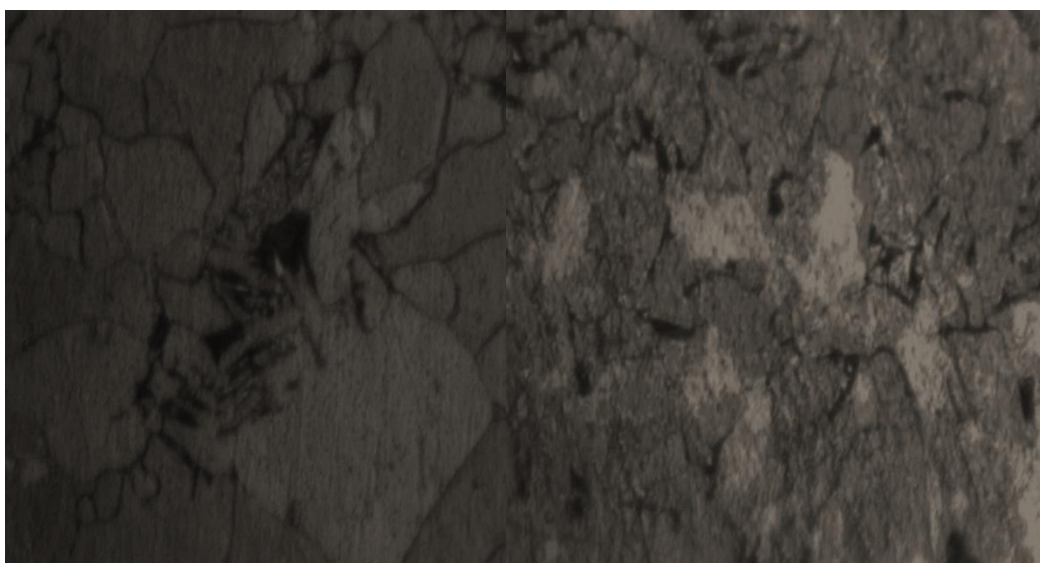
Plate III: Al7075/ 4wt% periwinkle ash composite Plate IV: Al7075/ 6wt% periwinkle ash composite
