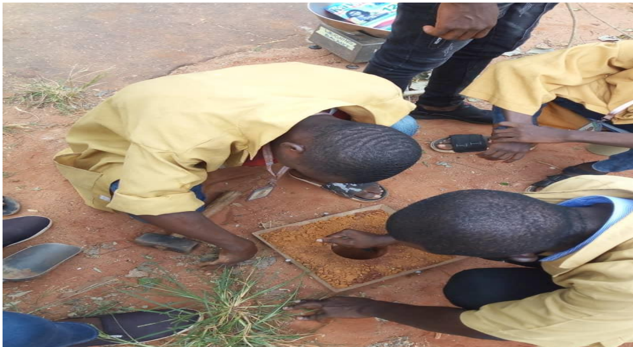
Figure 2: In-situ density test
