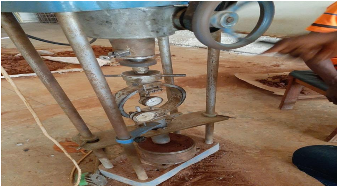
Figure 3: California bearing Ratio test being carried out in the laboratory
