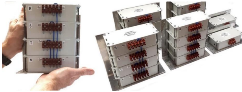
Fig. 18. Special HEMP filters designed by author for installation in current and voltage circuits of microprocessor-based protection relays
