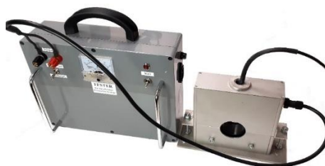
Fig. 22. Simple E3 component simulator for testing serviceability of the system for protection of high-power transformer
