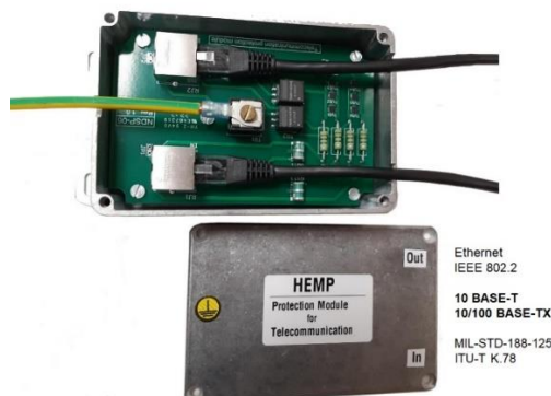
Fig. 26. HEMP protection module for telecommunications
