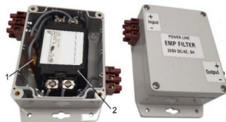
Fig. 19. HEMP power line filter for microprocessor-based protection relays inside the control cabinet. 1 – special high-efficiency surge arrester; 2 – electromagnetic two stage filter.
