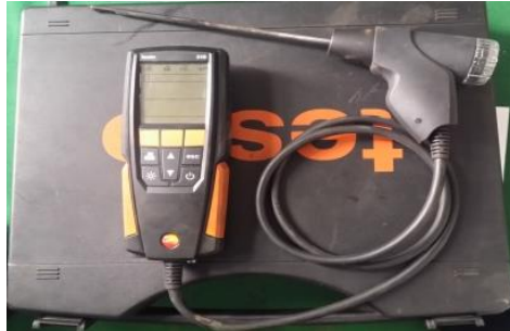
Figure 1: Flue gas analyzer-Testo 310
