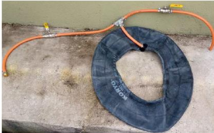
Fig 6: Raw gas storage tank assembly
