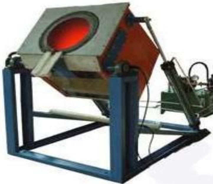
(a) 300 kg capacity high frequency induction furnace (b) Pouring of scrap-based molten 17-4 PH
