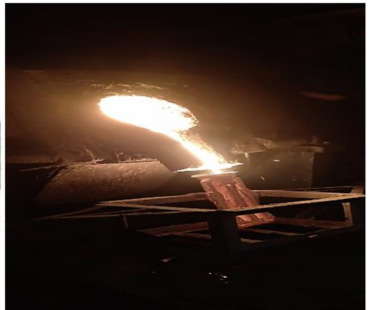
(a) 300 kg capacity high frequency induction furnace (b) Pouring of scrap-based molten 17-4 PH
