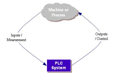
The PLC accepts inputs from switches and sensors (measures or senses the system), evaluates these based on a program (logic), and changes the state of outputs to control a machine or process.
