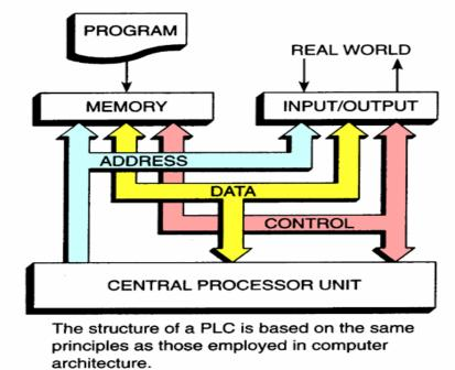
For the PLC to be useful, it must first have a Program or Logic for the CPU to execute. A system engineer or PLC programmer will first create the program logic in a programming device (these days it is usually software running on a personal computer). This logic can be written in Ladder Logic, Instruction List, Sequential Function Charts, or any of the IEC languages.
