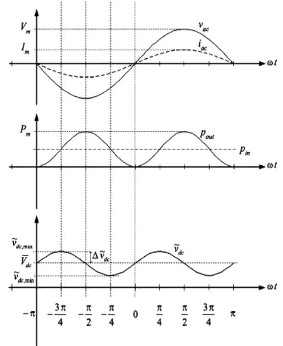
Fig. 3. Relationships among  $v_{ac}$ ,  $i_{ac}$ ,  $v_{dc}$ ,  $P_{in}$ , and  $P_{out}$ .
