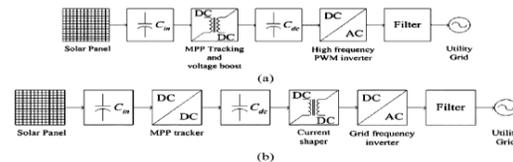
Fig. 1. Typical structures of grid-connected PV systems. (a) With voltage-fed, self-commutated inverter switching at high frequency. (b) With current-fed, grid-commutated inverter switching at the grid frequency.
