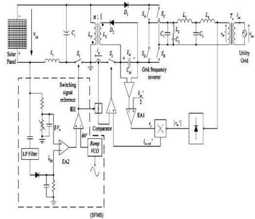
Fig. 2. Circuit schematics of the proposed inverter.
