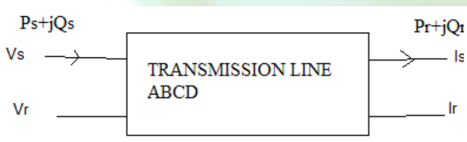
Figure 1. Two port four terminal model of a transmission line.
