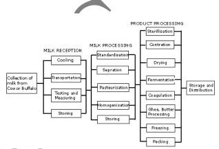
Fig.1-Block diagram of milk processing
