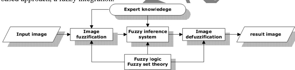
Fig-2: Structure of fuzzy image processing
