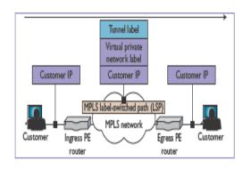
**Figure MPLS Tunneling Architecture**
