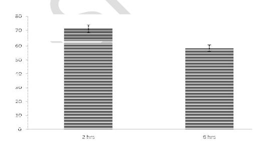
Figure 2. Effect of reaction times on biodiesel production. Bars indicate mean  $\pm$  SE (n = 3).
