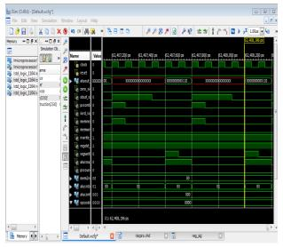
Fig.4. Shows Simulation Waveforms Add of Two 8-Bit Resisters Value
