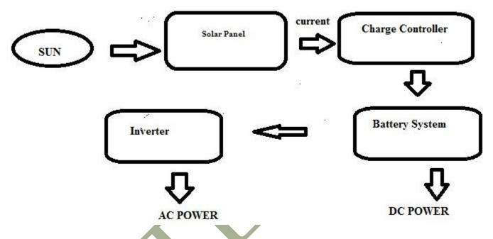
Figure 1.1 Showing process of solar energy
