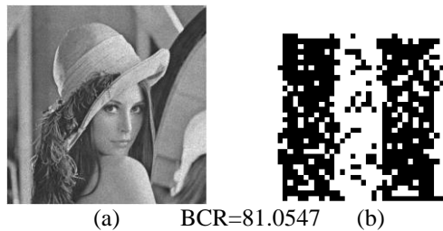
Figure 7: (a) Watermarked image attacked by salt & pepper noise. (b) Recovered watermark from watermarked image attacked by salt & pepper noise.
