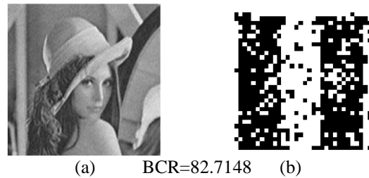
Figure 10: (a) JPEG compressed Watermarked image (compr coeff=5000). (b) Recovered watermark from JPEG compressed image with (compr coeff= 5000).
