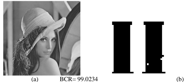
Figure 2: (a) cover image watermarked using DWT and D matrix of the SVD of the cover image. (b) Retrieved watermark.
