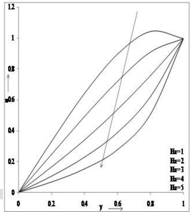
Figure 7. Velocity profiles versus  $y$  for different values of  $Ha$  when  $R=1, S=5.0, \omega=1.0, t=0.1, K_r=4.0, \lambda=0.1, \gamma=0.1, g=0.1, Pe=0.71, K=1.0, Gr=1.0, Gc=10, Sc=0.60, Re=2$ .
