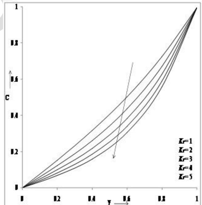
Figure 20. Concentration profiles versus  $y$  for different values of  $\Omega$  when  $R=1$ ,  $S=5.0$ ,  $t=0.1$ ,  $K_f=4.0$ ,  $\lambda=0.1$ ,  $\gamma=0.1$ ,  $g=0.1$ ,  $Pe=0.71$ ,  $K=1.0$ ,  $Ha=1.0$ ,  $Gr=1.0$ ,  $Gc=10$ ,  $Sc=0.60$ ,  $Re=2$ .
