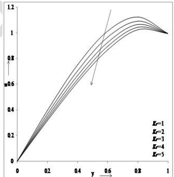
Figure 8. Velocity profiles versus  $y$  for different values of  $K_r$  when  $R=1, S=5.0, \omega=1.0, t=0.1, \lambda=0.1, \gamma=0.1, g=0.1, Pe=0.71, K=1.0, Ha=1.0, Gr=1.0, Gc=10, Sc=0.60, Re=2$ .
