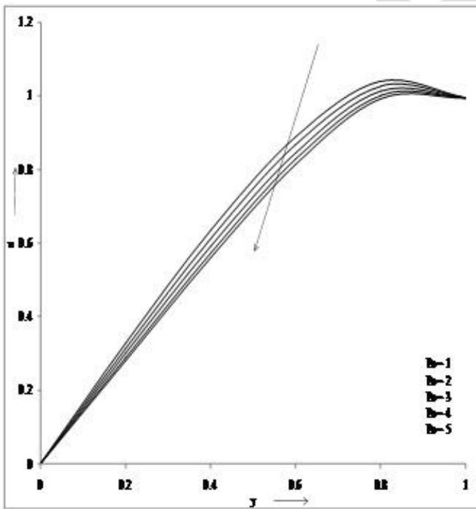
Figure 6. Velocity profiles versus  $y$  for different values of  $Pe$  when  $R=2, S=5.0, \omega=1.0, t=0.1, K_r=4.0, \lambda=0.1, \gamma=0.1, g=0.1, K=2.0, Ha=2.0, Gr=1.0, Gc=1, Sc=0.60, Re=2$ .
