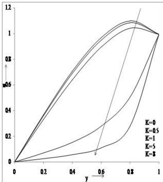
Figure 9. Velocity profiles versus  $y$  for different values of  $K$  when  $R=1, S=5.0, \omega=1.0, t=0.1, K_r=4.0, \lambda=0.1, \gamma=0.1, g=0.1, Pe=0.71, Ha=1.0, Gr=1.0, Gc=10, Sc=0.60, Re=2$ .
