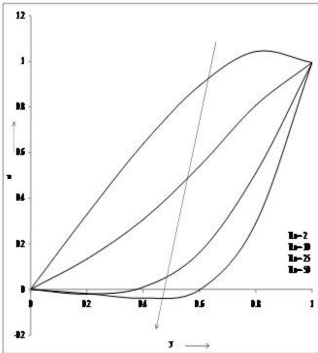
Figure 5. Velocity profiles versus  $y$  for different values of  $Re$  when  $R=1, S=5.0, \omega=1.0, t=0.1, K_r=4.0, \lambda=0.1, \gamma=0.1, g=0.1, Pe=0.71, K=1.0, Ha=1.0, Gr=1.0, Gc=10, Sc=0.60$ .
