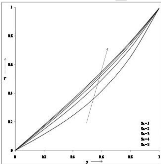
Figure 18. Concentration profiles versus  $y$  for different values of  $Sc$  when  $R=1$ ,  $S=5.0$ ,  $\omega=1.0$ ,  $t=0.1$ ,  $K_f=4.0$ ,  $\lambda=0.1$ ,  $\gamma=0.1$ ,  $g=0.1$ ,  $Pe=0.71$ ,  $K=1.0$ ,  $Ha=1.0$ ,  $Gr=1.0$ ,  $Gc=10$ ,  $Re=2$ .
