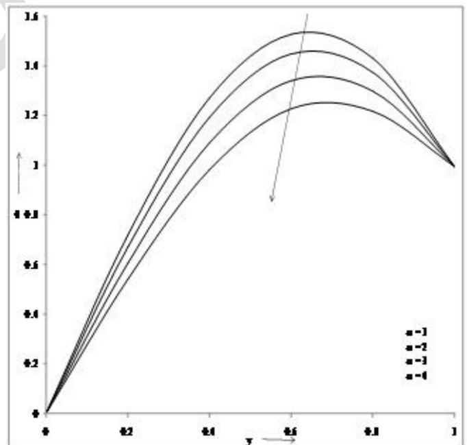
Figure 16. Temperature profiles versus  $y$  for different values of  $\omega$  when  $R=1$ ,  $S=5.0$ ,  $t=0.1$ ,  $K_r=4.0$ ,  $\lambda=0.1$ ,  $\gamma=0.1$ ,  $g=0.1$ ,  $Pe=0.71$ ,  $K=1.0$ ,  $Ha=1.0$ ,  $Gr=1.0$ ,  $Gc=10$ ,  $Sc=0.60$ ,  $Re=2$ .
