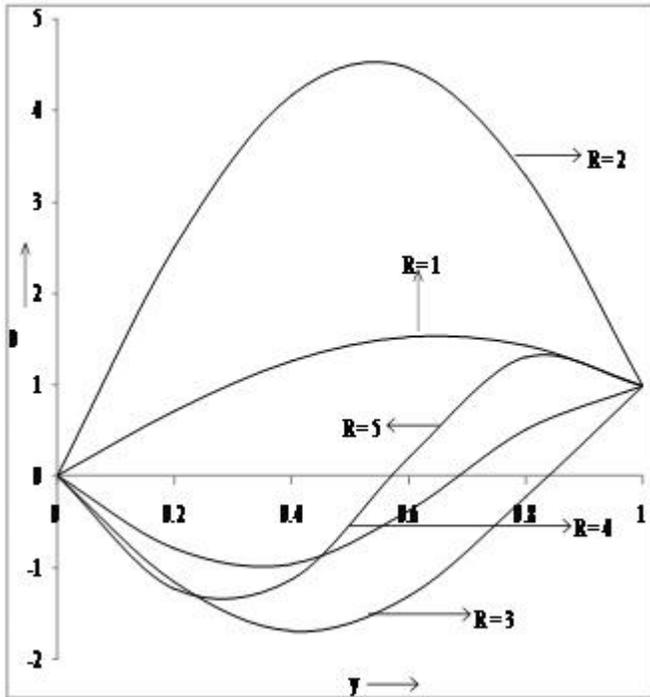
Figure 17. Temperature profiles versus  $y$  for different values of  $R$  when  $S=5.0$ ,  $\omega=1.0$ ,  $t=0.1$ ,  $K_f=4.0$ ,  $\lambda=0.1$ ,  $\gamma=0.1$ ,  $g=0.1$ ,  $Pe=0.71$ ,  $K=1.0$ ,  $Ha=1.0$ ,  $Gr=1.0$ ,  $Gc=10$ ,  $Sc=0.60$ ,  $Re=2$ .
