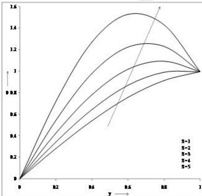
Figure 14. Temperature profiles versus  $y$  for different values of  $S$  when  $R=1$ ,  $\omega=1.0$ ,  $t=0.1$ ,  $K_r=4.0$ ,  $\lambda=0.1$ ,  $\gamma=0.1$ ,  $g=0.1$ ,  $Pe=0.71$ ,  $K=1.0$ ,  $Ha=1.0$ ,  $Gr=1.0$ ,  $Gc=10$ ,  $Sc=0.60$ ,  $Re=2$ .
