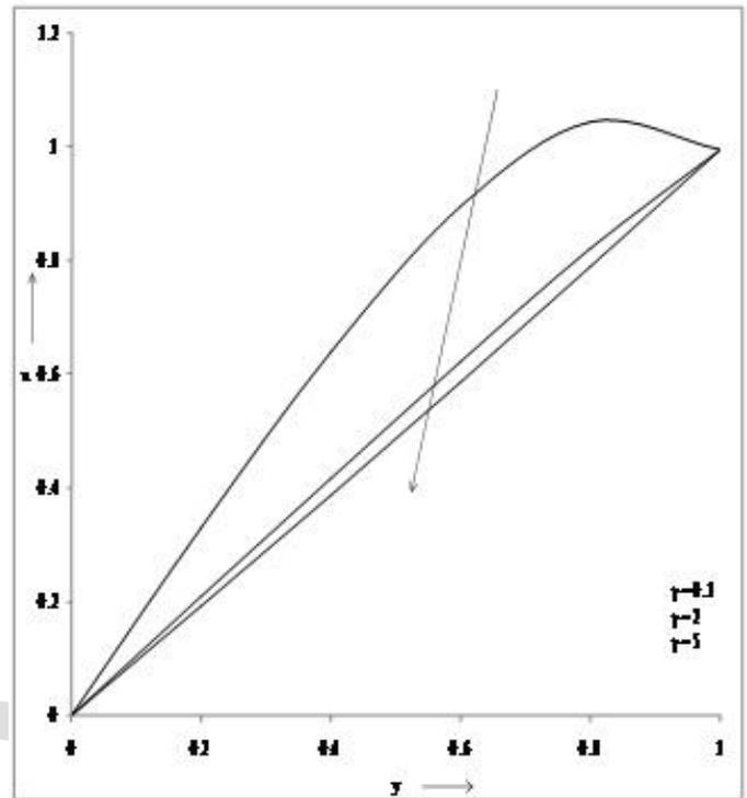
Figure 11. Velocity profiles versus  $y$  for different values of  $\gamma$  when  $R=1, S=5.0, \omega=1.0, t=0.1, K_r=4.0, \lambda=0.1, g=0.1, Pe=0.71, K=1.0, Ha=1.0, Gr=1.0, Gc=10, Sc=0.60, Re=2$ .
