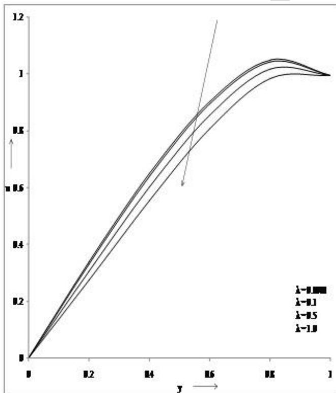
Figure 10. Velocity profiles versus  $y$  for different values of  $\lambda$  when  $R=1, S=5.0, \omega=1.0, t=0.1, K_r=4.0, \gamma=0.1, g=0.1, Pe=0.71, K=1.0, Ha=1.0, Gr=1.0, Gc=10, Sc=0.60, Re=2$ .
