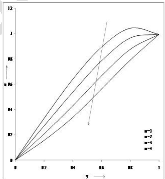
Figure 12. Velocity profiles versus  $y$  for different values of  $\omega$  when  $R=1, S=5.0, t=0.1, K_r=4.0, \lambda=0.1, \gamma=0.1, g=0.1, Pe=0.71, K=1.0, Ha=1.0, Gr=1.0, Gc=10, Sc=0.60, Re=2$ .
