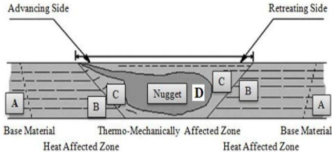
Figure-2: Schematic diagram of micro structural zones in friction stir welds in aluminium
