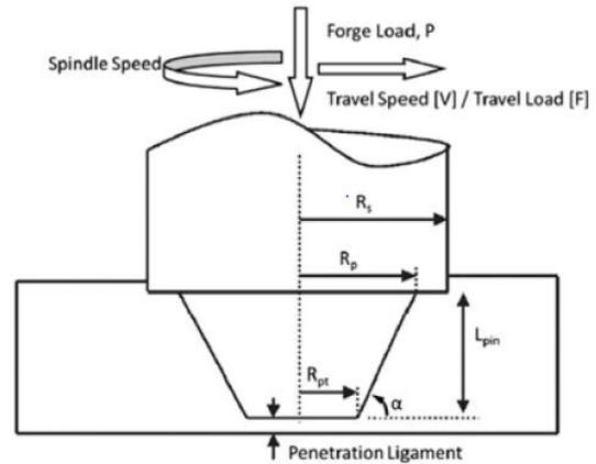
Figure.4 : Basic geometry for a FSW tool [23]
