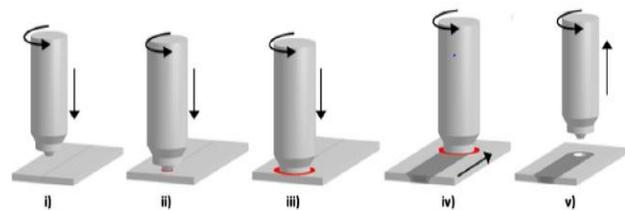
Figure. 5: FSW process steps [24].
