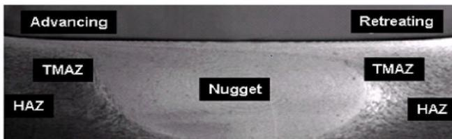
Figure 3: micrograph showing various micro-structural zones [Threadgill 1999][7]
