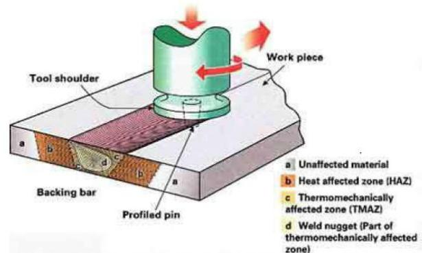
**Figure-1:** Friction stir welding principle and microstructure
