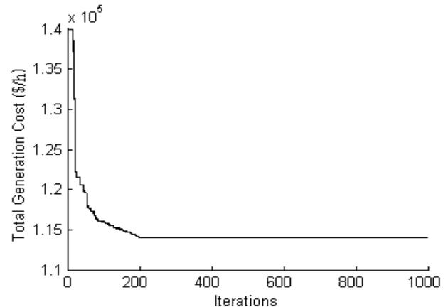
Fig.4. Convergence profile of the total generation cost for the test system1
