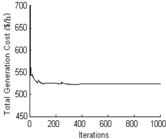
Fig.5. Convergence profile of the total generation cost for the test system 2.
