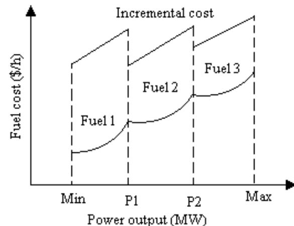
Fig. 2. Piecewise quadratic and incremental cost function of a generator.
