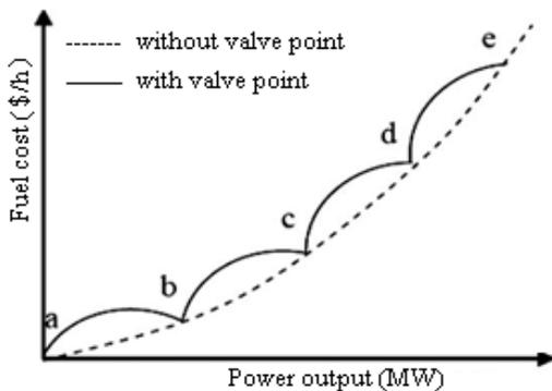
Fig. 1. Input-output curve with valve-point effects: a, b, c, d, e-valve points
