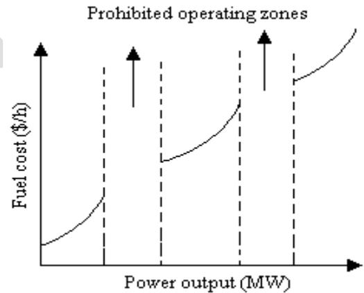
Fig. 3. Input-output curve with prohibited operating zones.
