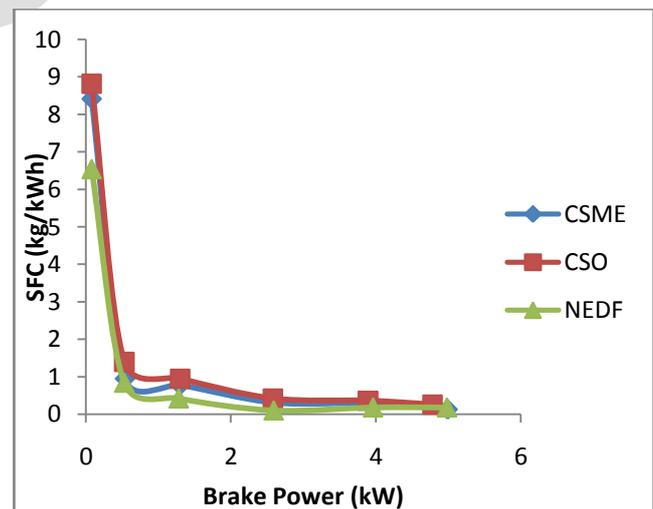
Fig. 2. Variation of SFC with brake power
