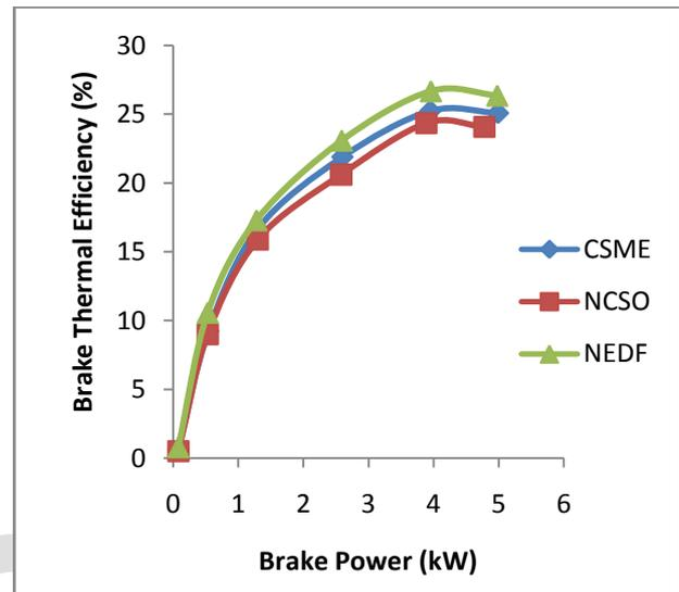
Fig. 1. Variation of brake thermal efficiency with brake power
