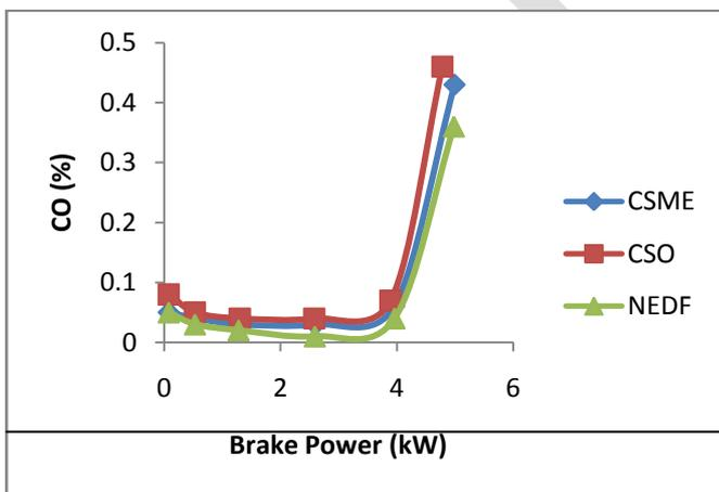
Fig. 4. Variation of CO with brake power
