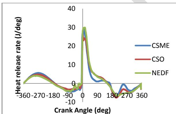
Fig.8. Variation of heat release rate with crank angle
