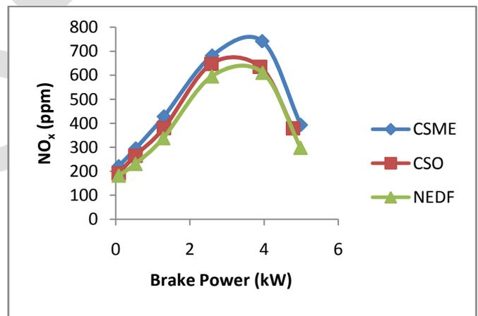
Fig. 6. Variation of NOx with brake power
