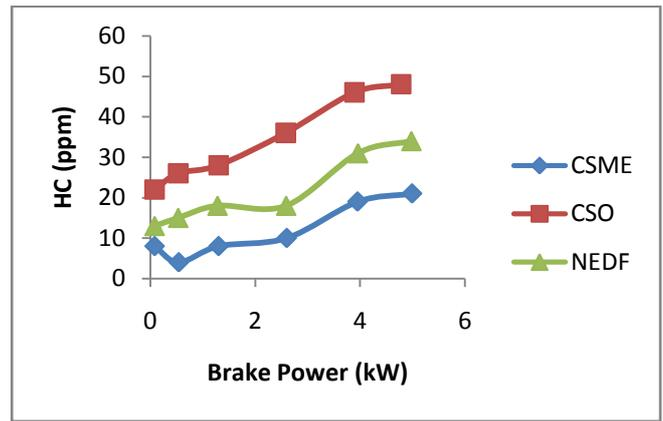
Fig.5. Variation of Hydrocarbon with brake power
