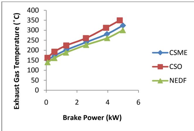
Fig. 3. Variation of EGT with brake power
