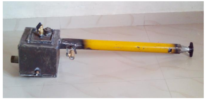
Fig.5 Vapor Fuel Injection with Help of Bubbler Kit
