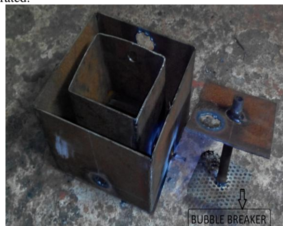
Fig.3 Inside view of bubbler
