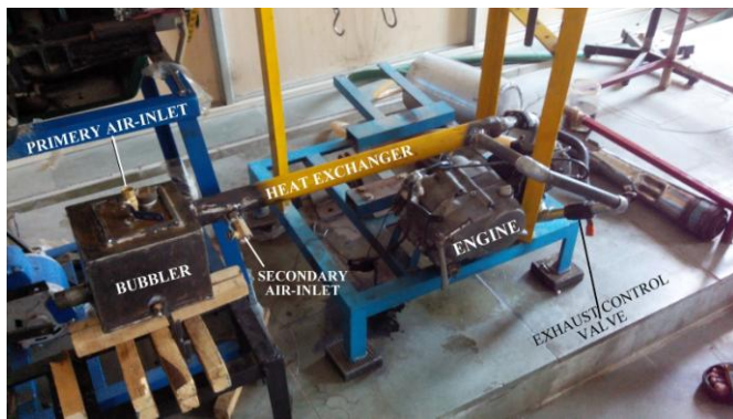
Fig.7 Experimental Set-up for vapor fuel system
