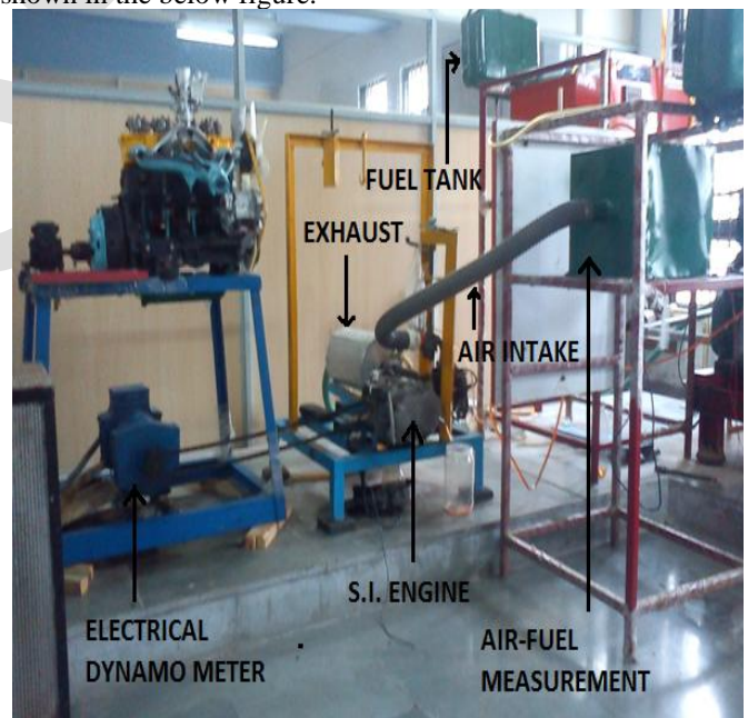
Fig.6 Experimental Set-up for carburettor system
