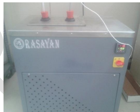
Figure 1: Cloud point and Pour point apparatus, Rasayan Make
