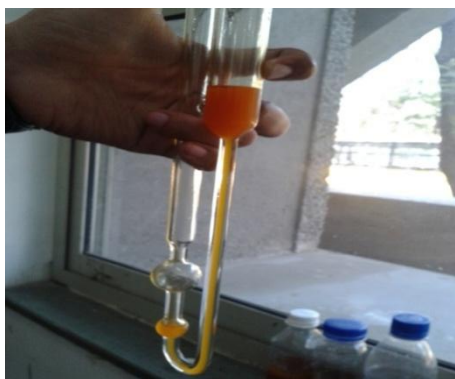
Figure 2: Reverse flow tube viscometer
