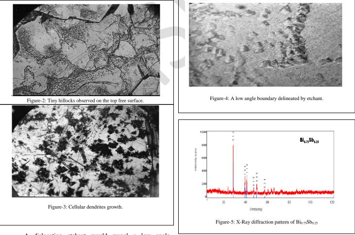
A dislocation etchant would reveal a low angle boundary on a crystal. In the present case a low angle boundary delineated by this etchant is shown in the Figure-4. Some of the
