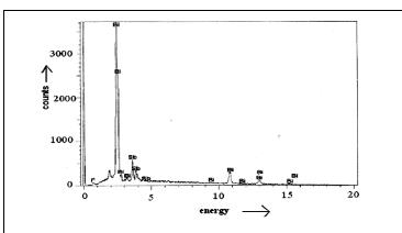
Fig.-6. Compositional analysis's of Bi  $_{0.75}$  Sb  $_{0.25}$  crystal, by EDAX
