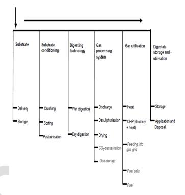
Figure 2. Process steps of biogas technologies
