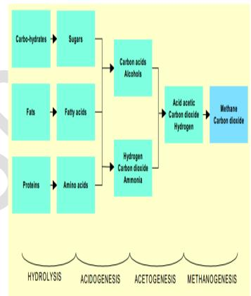
Figure-1.The simplified diagram of the AD process
