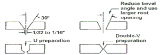
Figure 13. Edge-preparation and fit-up
