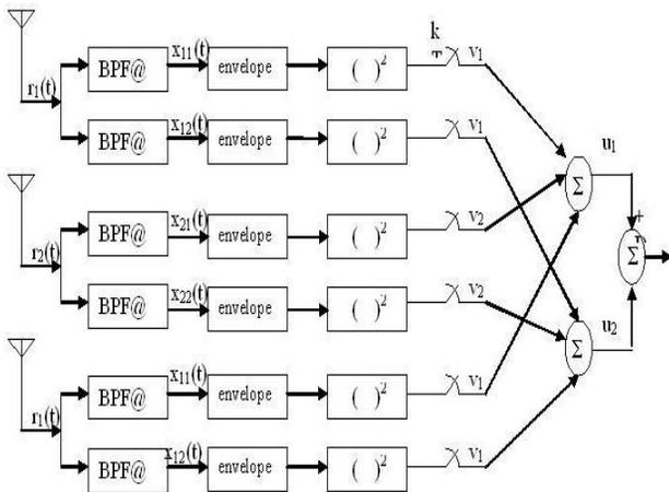
Fig. 1. Postdetection combiner for FSK
