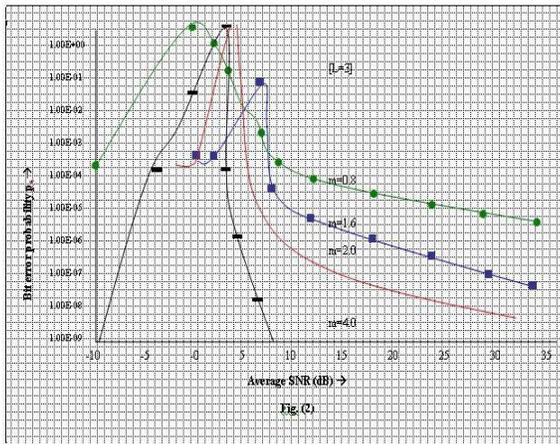
Fig. 2. Variation of Pe with SIR for m=0.8, 1.6, 2, 4 for L=3
