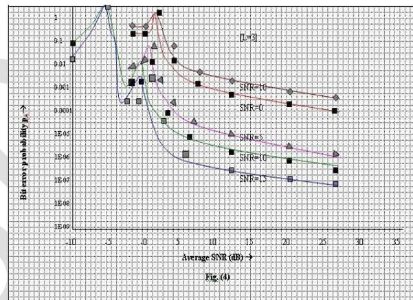
Fig. 4. Variation of Pe with SIR for SNR=-10dB, 0 dB, 5dB, 10dB and 15 dB for L=3
