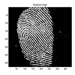
Here the above figure 1 is the input image and figure 2 is the image after equalization. Both the images shows the changes in the input image and the equalized image as the figure 2 is more clear than the input image.
