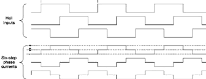
Fig.3 120-degree modulation and commutation
