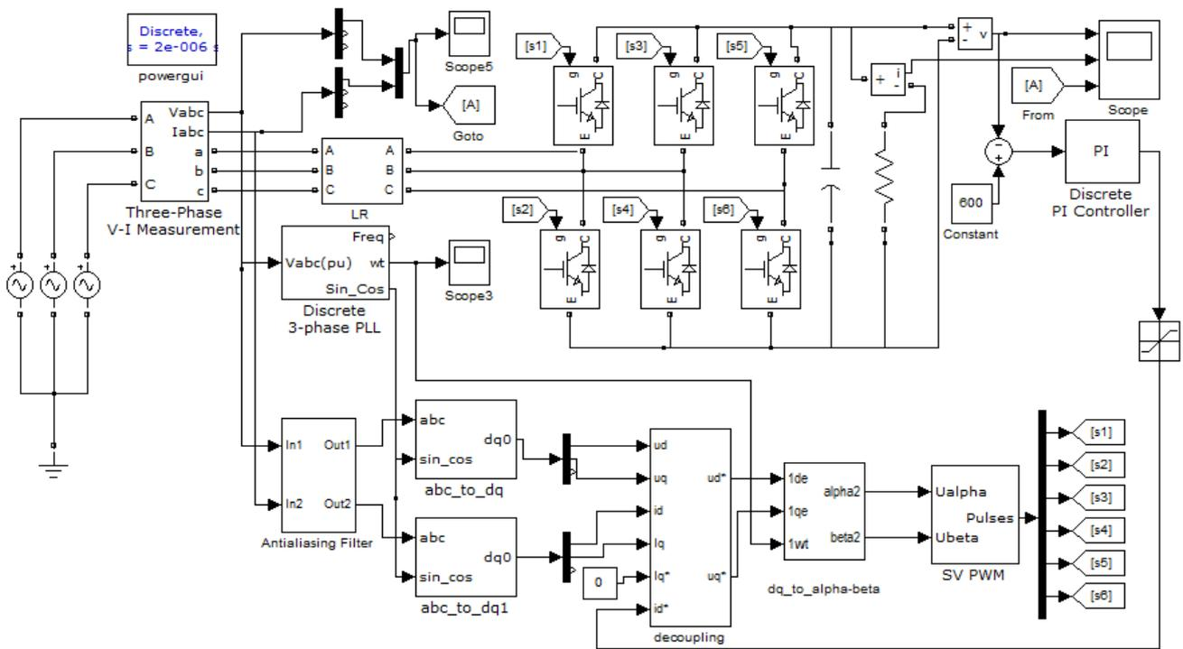
Fig. 5. Simulation model of 3-φ voltage source PWM rectifier in MATLAB/SIMULINK
