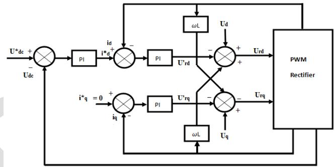
Fig. 2. Dual close-loop controller for PWM rectifier
