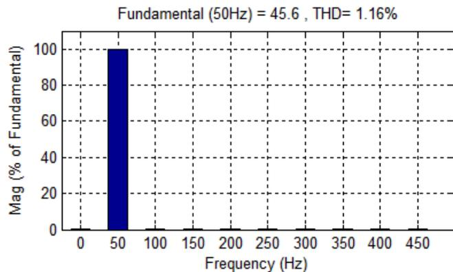
Fig. 8 FFT analysis of input current
