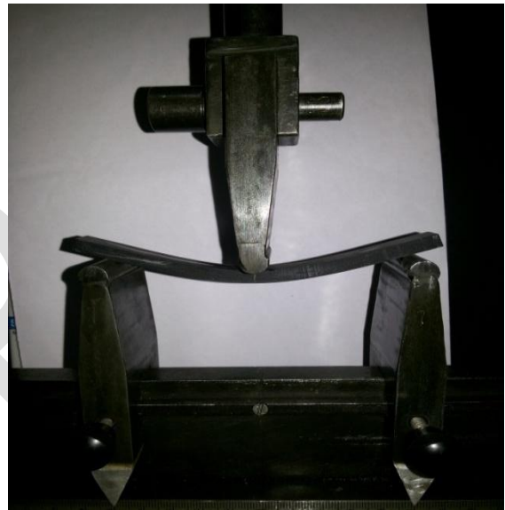
Figure 3: Position of test specimen for flexural test
