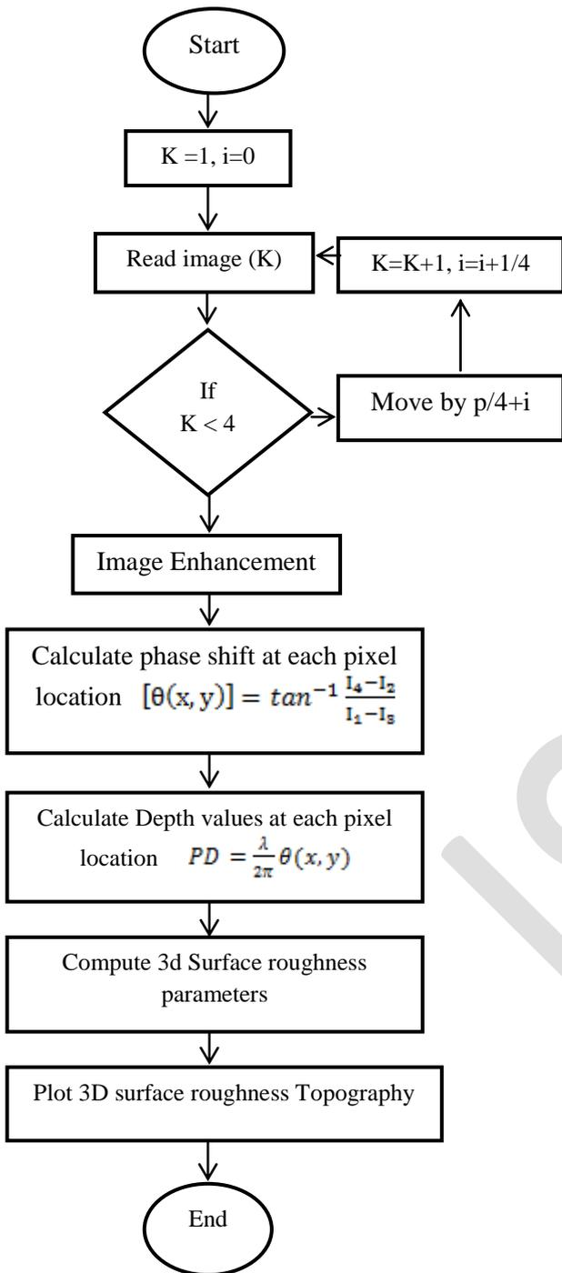
Fig. 3 Flow chart showing experimentation procedure
