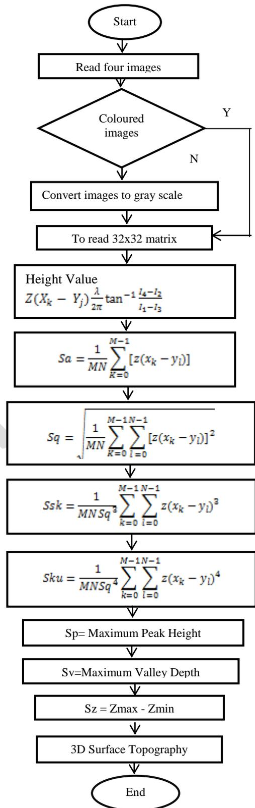
Fig. 4 Flow chart for developed algorithm for 3D surface roughness parameter measurement
