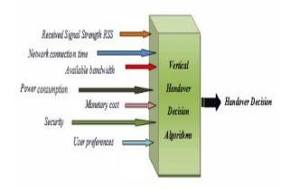
Fig 1. Parameters used for making YHD decision
