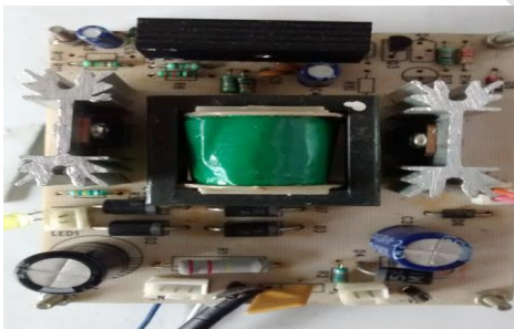
Fig. 14. 100W SEPIC MPPT converter
