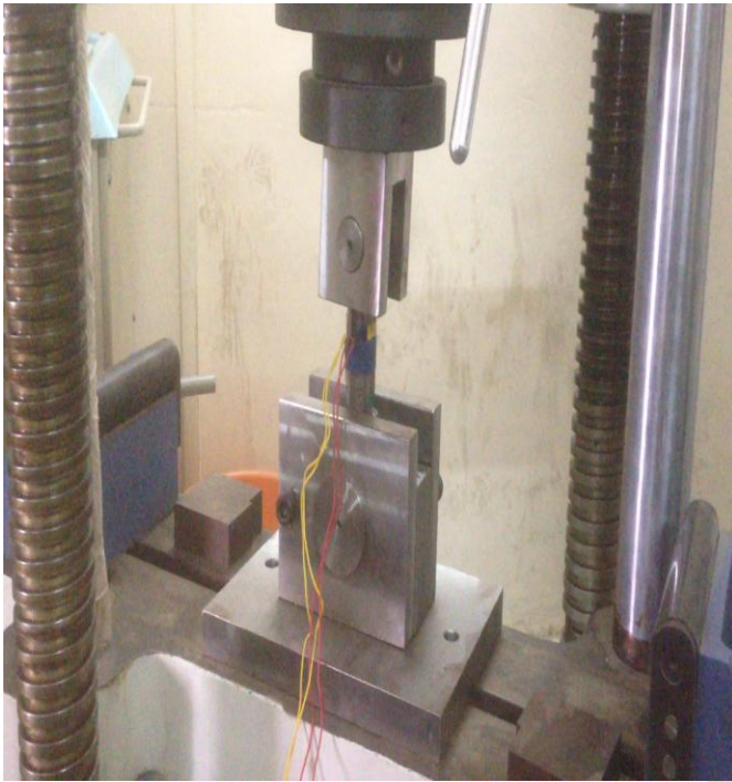
Fig. 2 Arrangement of fixture for holding connecting rod
