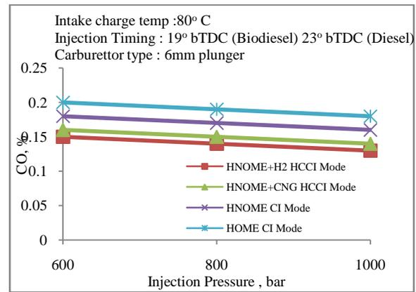
Fig. 6 Variation CO with Injection pressure
