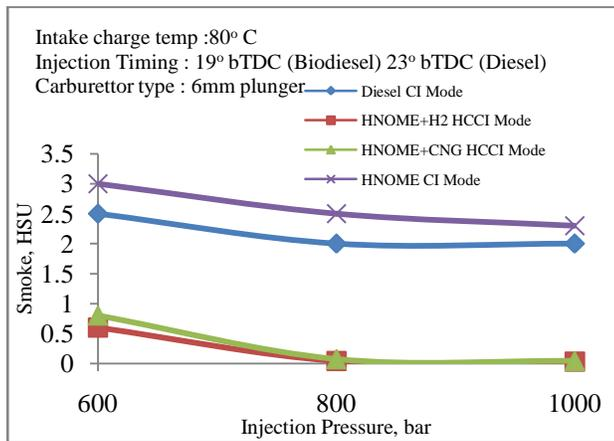
Fig. 8 Variation Smoke with Injection pressure
