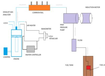
Fig. 3 Schematic representation of the experimental set up used to collect HCCI data
