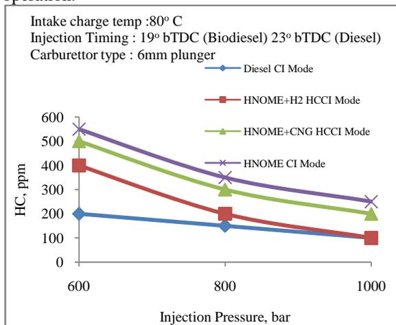
Fig. 5 Variation HC with Injection pressure
