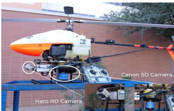
Fig2. Architecture of an unmanned aircraft
