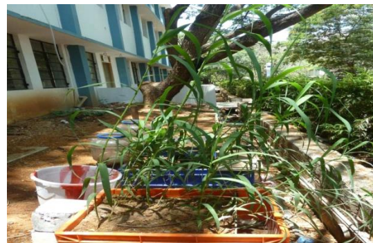
Fig.3 (b) Final stages of wetland unit tub with phragmites Australis
