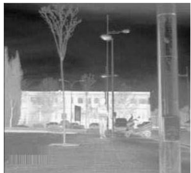
Fig.1 A thermal video frame where the moving object is undetectable due to the glass pane before the target.
