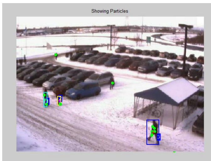
Fig.7 Video frame with multiple targets wherein the results obtained by visible camera are more discriminatory than the thermal camera.
