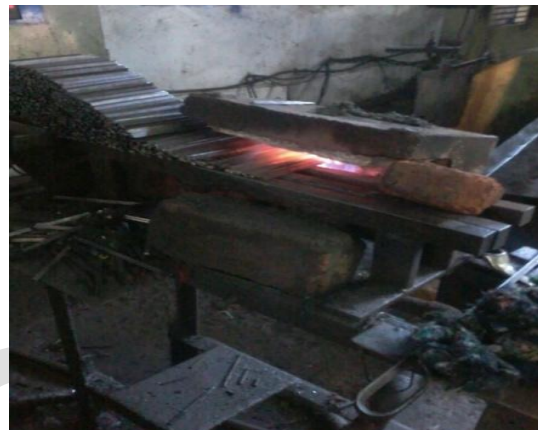
Figure No-07:Tang Forging Set Up with Gas Fired Furnace
