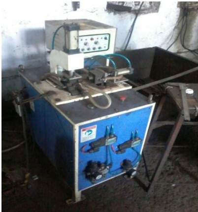
Figure No-08:Tang Forging Set Up with Special Purpose Resistance Heating Furnace
