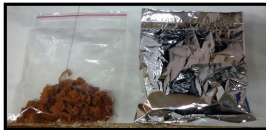
Fig 3. Snack food packed in LDPE and Metallised Polyester.
