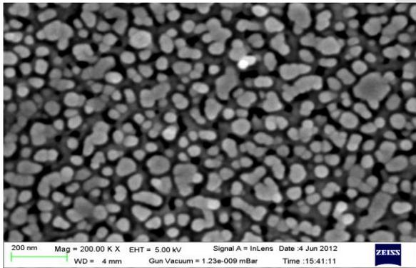
Fig. 3: FESEM image of ZnO thin films grown on quartz substrates by sol gel spin coating method.
