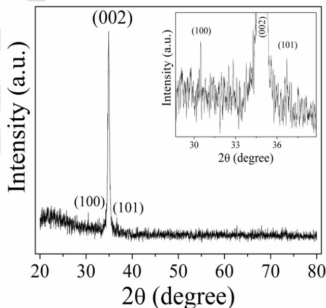
Fig. 1: X-ray diffraction pattern of indium doped ZnO thin film in the  $2\theta$  range (20-80) degree. Inset shows the magnified image of diffraction peaks.
