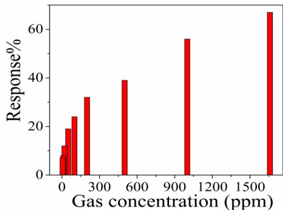
Fig. 5: Variation of response% of indium doped ZnO thin film towards the detection of various concentrations of CO gas at their optimum temperature, 350°C
