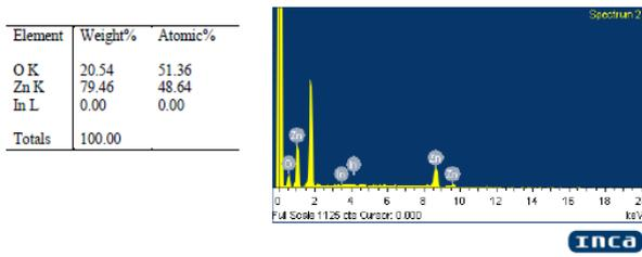
Fig.2: EDs measurement of indium doped ZnO thin films showing no other impurity phases
