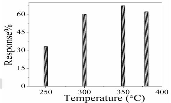
Fig. 4: Variation of response% of indium doped ZnO thin film towards the detection of 1660 ppm of CO gas as a function of operating temperature
