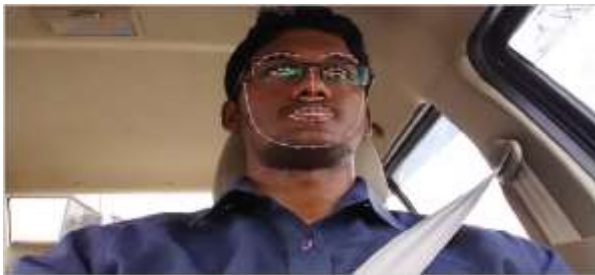
Fig. 2. Sample frame marked with 66 facial AAM landmarks
