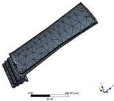
Fig. 2 Turbine blade with meshed
