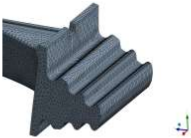
Fig. 3 Turbine root of blade meshed
